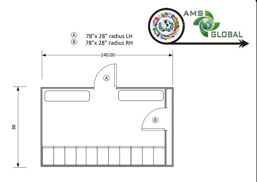
All metal and composite construction LED 100,000 hour burn lighting 240 VAC power requirement 13,500 BTU AC with 5500 watts heat Dusk till dawn porch light Motion activated interior lighting Ten 12"x18"x72" lockers Two built in 4' benches Broom and mechanical storage Sky light door
