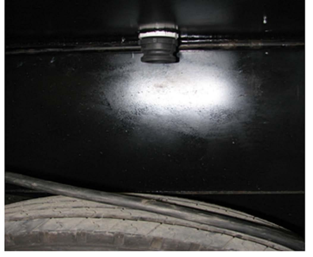
The pump out valve should connected to the 2" cam-lock should never be opened unless it is connected to a pump truck, external holding tank, or directly to a septic or sewer system.
